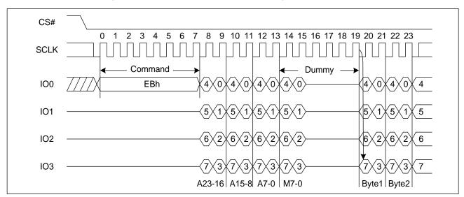
Figure 16. Quad I/O Fast Read Sequence Diagram ((M5-4) ≠ (1, 0))
