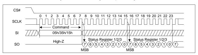
Figure 7. Read Status Register Sequence Diagram
