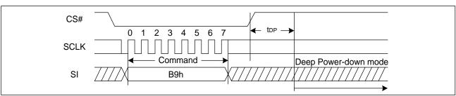
Figure 34. Deep Power-Down Sequence Diagram
