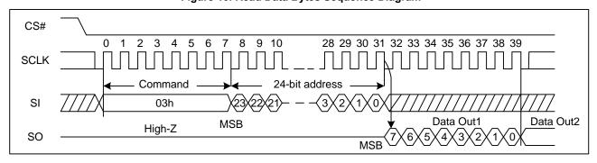
Figure 10. Read Data Bytes Sequence Diagram
