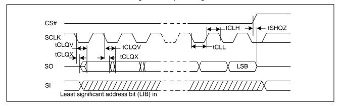
Figure 43. Resume to Suspend Timing Diagram
