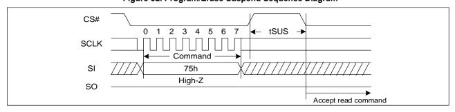
Figure 32. Program/Erase Suspend Sequence Diagram
