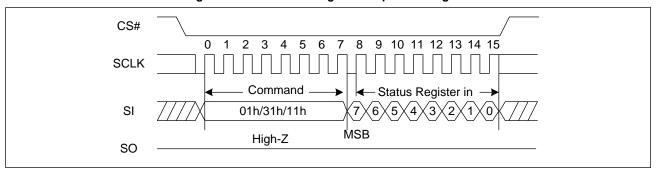
Figure 8. Write Status Register Sequence Diagram
