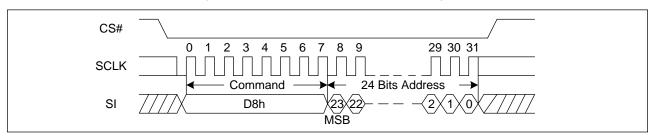
Figure 23. 64KB Block Erase Sequence Diagram
