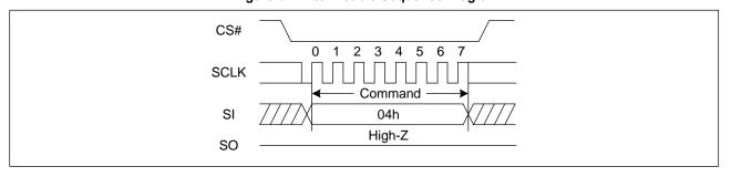
Figure 6. Write Disable Sequence Diagram
