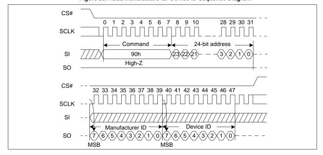
Figure 25. Read Manufacture ID/ Device ID Sequence Diagram
