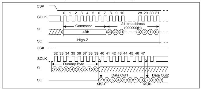
Figure 27. Read Unique ID Sequence Diagram
