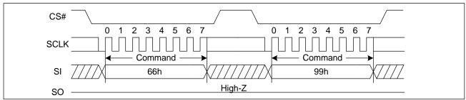
Figure 31. Enable Reset and Reset command Sequence Diagram
