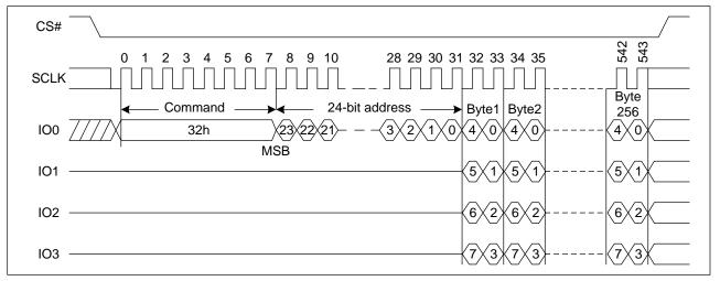
Figure 20. Quad Page Program Sequence Diagram
