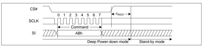
Figure 35. Release Power-Down Sequence Diagram
