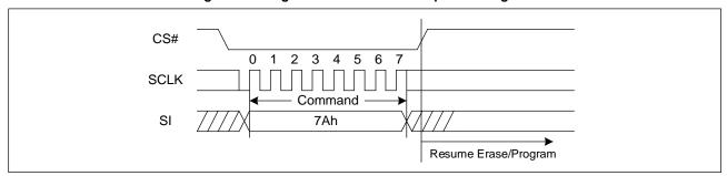
Figure 33. Program/Erase Resume Sequence Diagram
