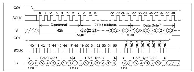
Figure 29. Program Security Registers command Sequence Diagram
