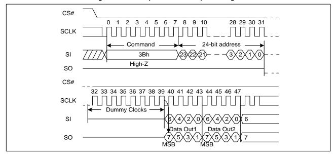
Figure 12. Dual Output Fast Read Sequence Diagram
