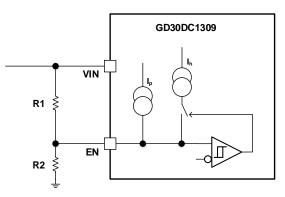
Figure 4. PVIN UVLO Setting (VIN≥4.5V)
