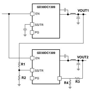
Figure 15. Ratiometric and Simultaneous Start-Up Sequence
