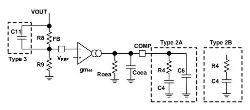
Figure 10. Types of Frequency Compensation
