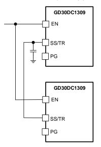
Figure 14. Ratiometric Start-Up Sequence
