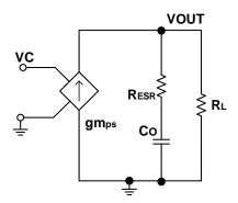
Figure 8. Small Signal Model for Loop Response
