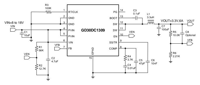
Figure 16. 3.3V, 6A Reference Design
