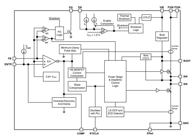
Figure 1. GD30DC1309 Functional Block Diagram
