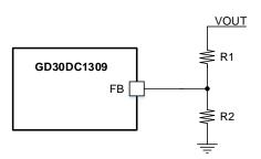
Figure 2. Feedback resistor divider diagram
