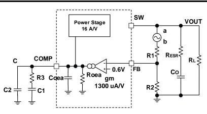
Figure 7. Small Signal Model for Loop Response
