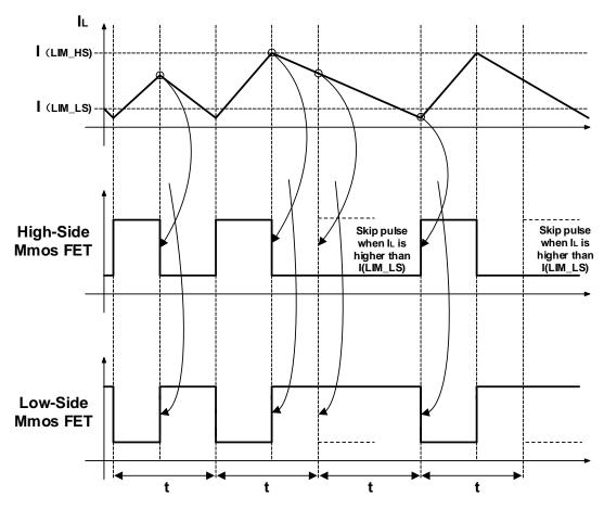
Figure 6. Overcurrent Protection for Both MOSFETs
