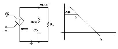
Figure 9. Small Signal Model for Loop Response
