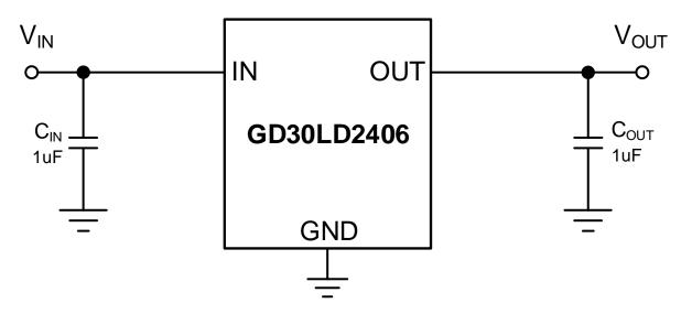
Figure 2. Reference Design Schematic
