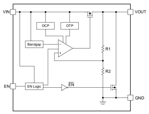
Figure 1. GD30LD2406 Functional Block Diagram
